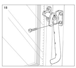
Finally, mark out screw holes on the frame to ensure correct positioning of the fitting as compared with the bar part.
