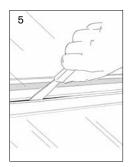
**Glazing bars:** Insert a putty knife behind the internal cover cap (4), move it along the glazing bar (5) and detach the cover cap.
