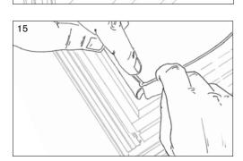
Press the glazing gasket in, starting at the corners and then proceeding on the sides. Be careful not to twist the gasket.
