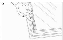
Press the glazing bead loose and pull it out (8).
