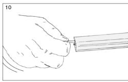
Mark out screw holes on the glazing bead in accordance with the installation drawing.
