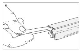
Push the pressure distribution plate 8cm up at the bottom of the glazing bead using a long, thin screwdriver or the like.
