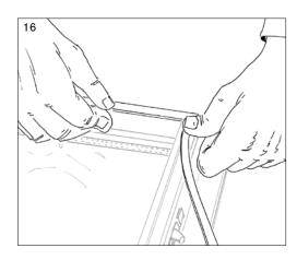
Attach the weather strip, starting at the top, then proceed to the corners and sides.
