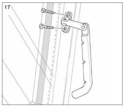
Fasten the bar part of the PN-fitting using four 13mm screws.
